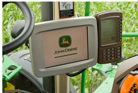
Dual display configuration with the mobile processor removed on the Original GreenStar System.
