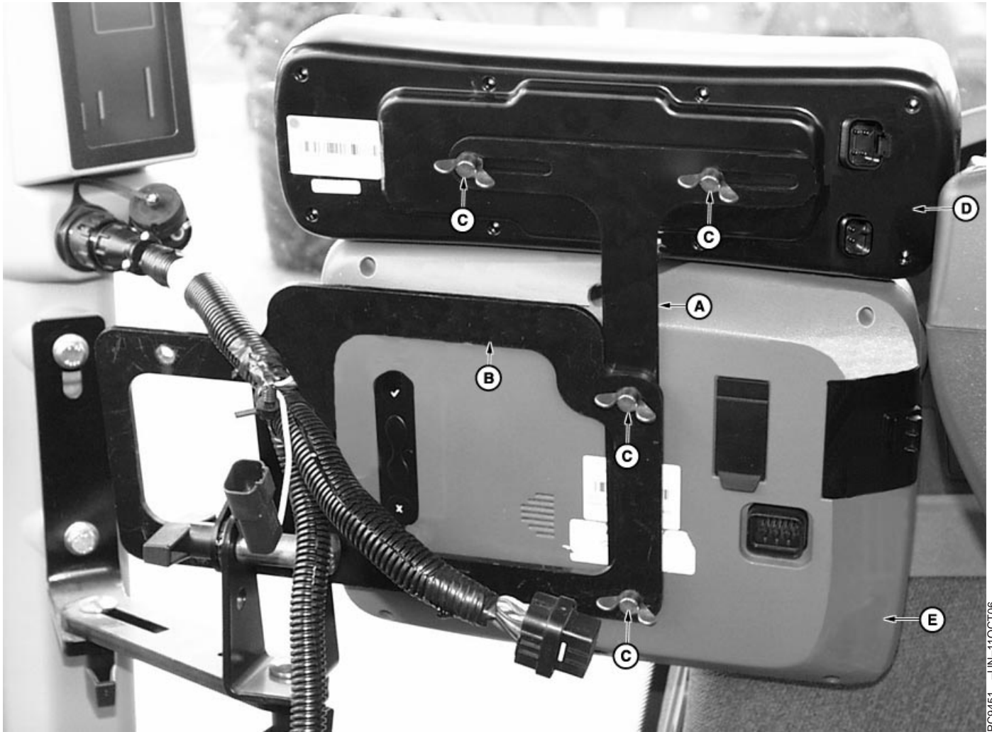
Installing Switch Box
