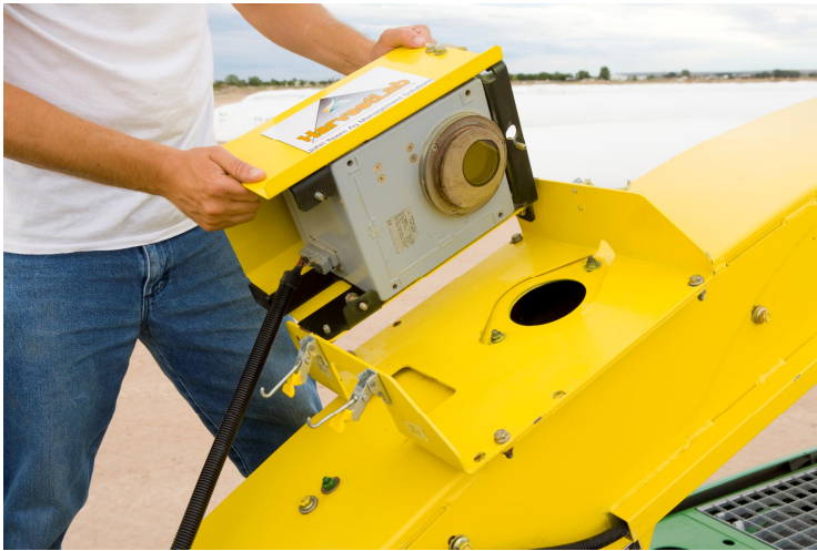
HarvestLab™ moisture sensor mounted on an SPFH spout
