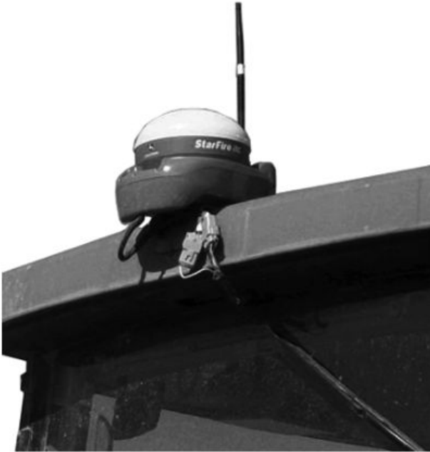
RTK Receiver on Top of Cab
